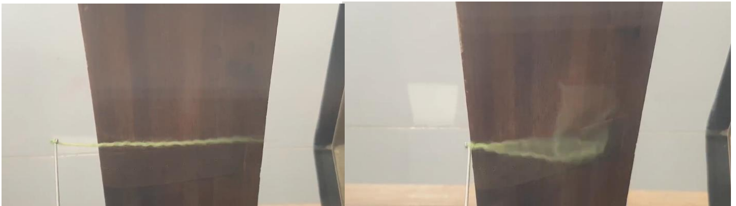
Figure 8 - Comparison of flow attachment vs separation
