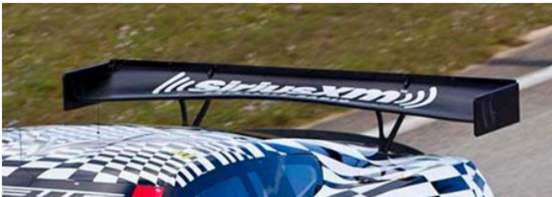
Figure 33 - Corvette C7.R twisted wing(Racecar Engineering, 2015)
