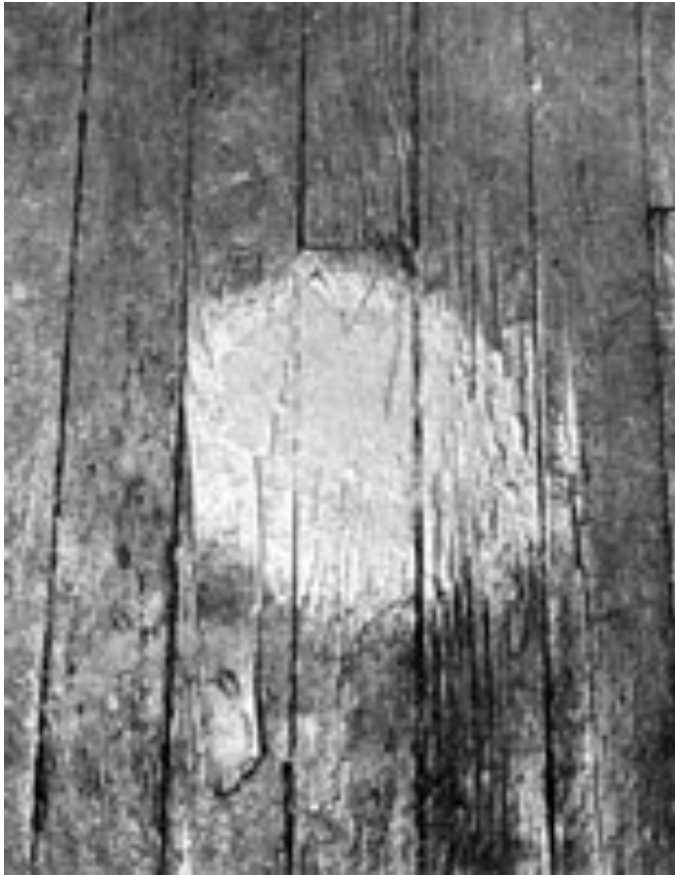
Gloss White Lacquer Sprayed For 2 Minutes At Forty Pound Pressure Directly Upon The Floor
