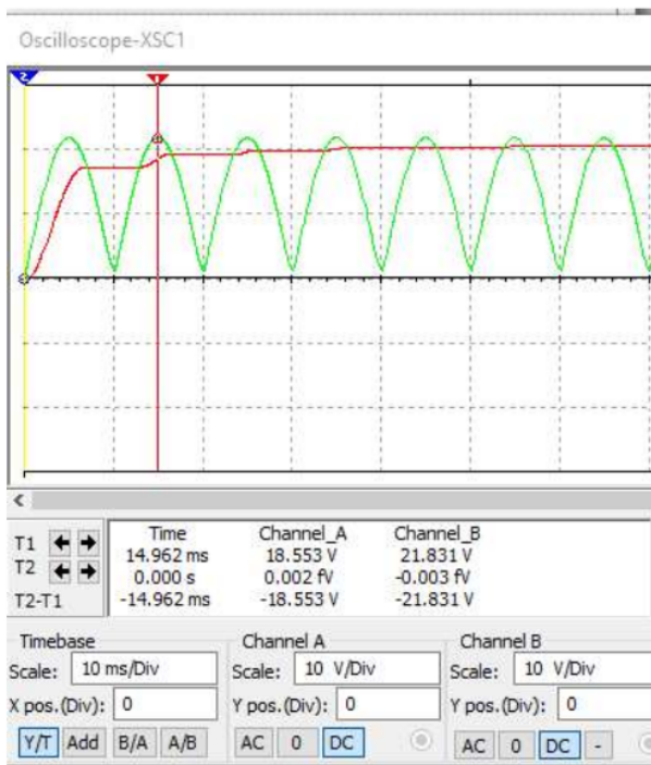
Figure 24 – Rectified Voltage compared with Voltage Across Capacitor
