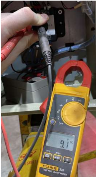
Figure 34 – 9V when PS2 Switched
