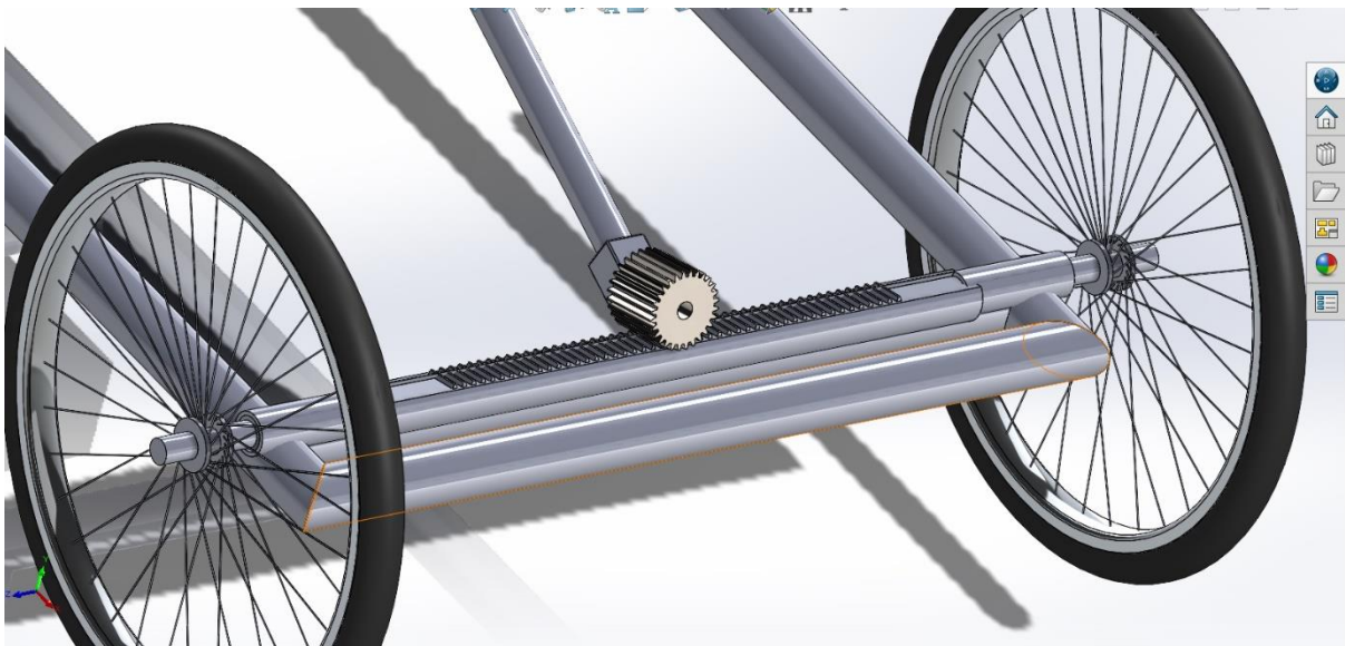
Figure 4 - Figure 4 - Close up of the rack and pinion steering system (Aganon, 2022)
