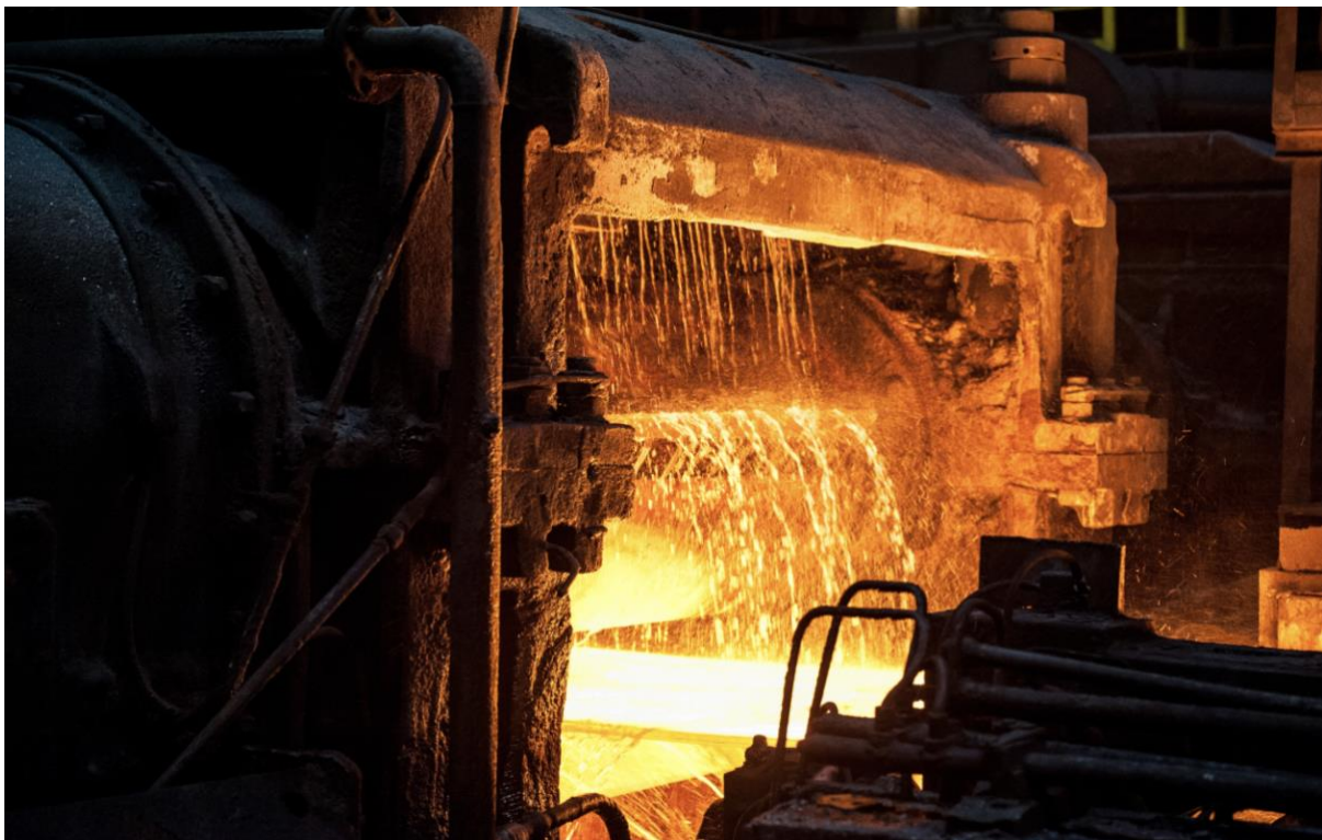
Figure 16 - Steel Slab being 'Descaled' Through the HSB/VSB
