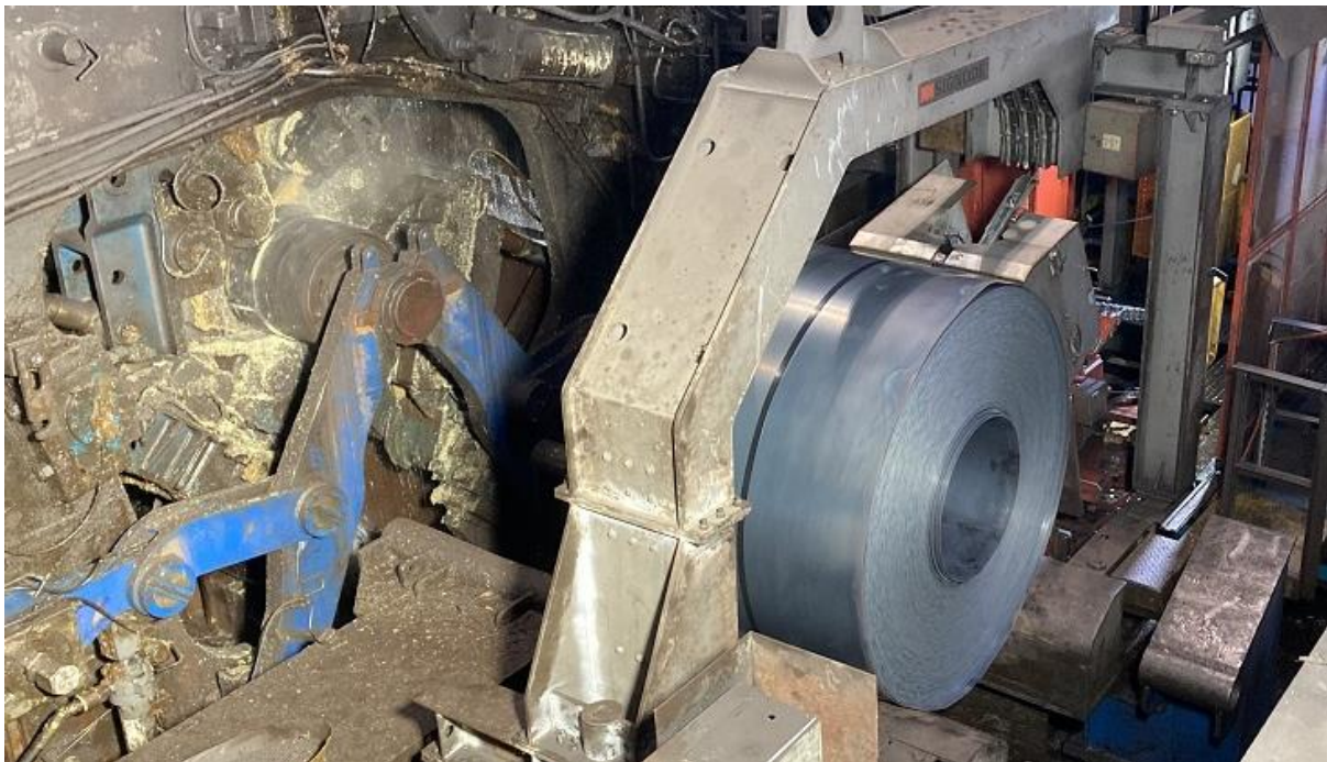
Figure 27 - Hot Rolled Coil (HRC) exiting the down coilers
