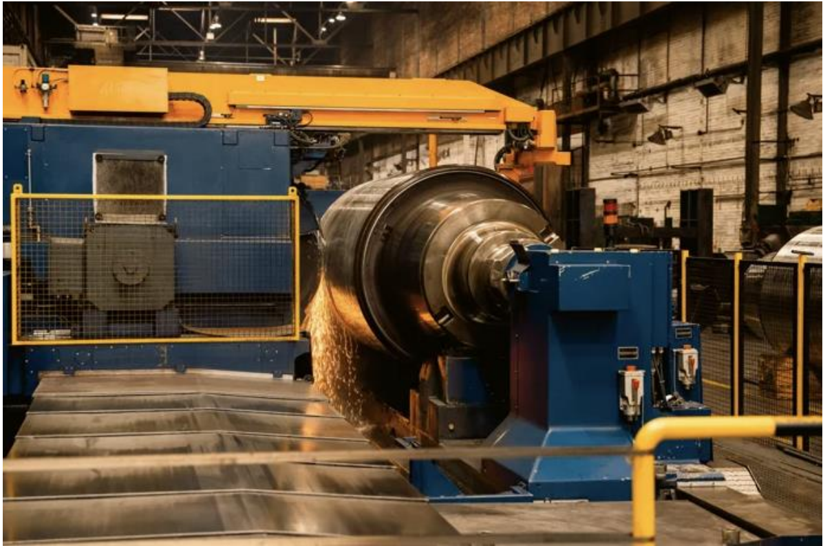
Figure 30 - Back up roll being ground before reinsertion in the roughing mill
