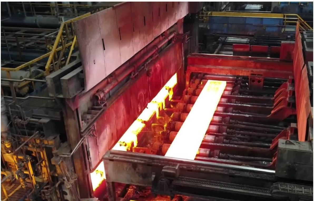
Figure 15 - Heated Steel Slab being Discharge from Reheat Furnace A
