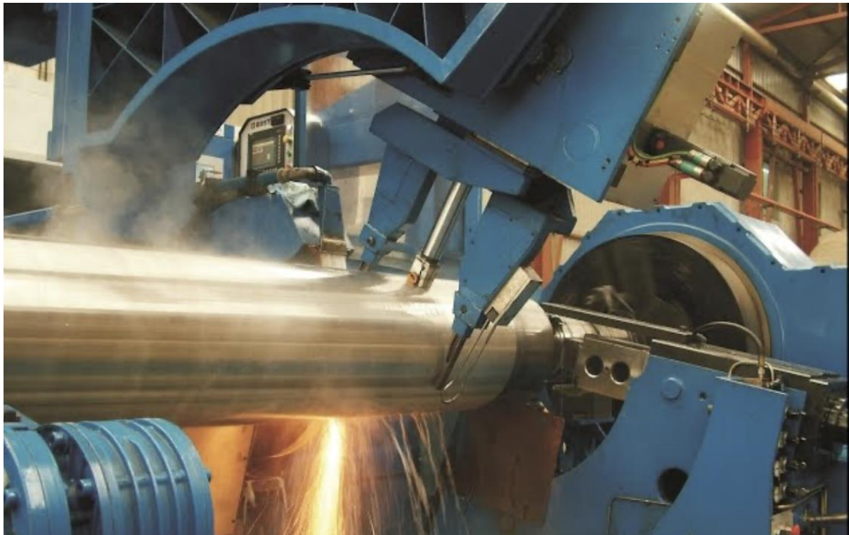
Figure 29 - Work Roll being ground before being reused in the Finishing Stands
