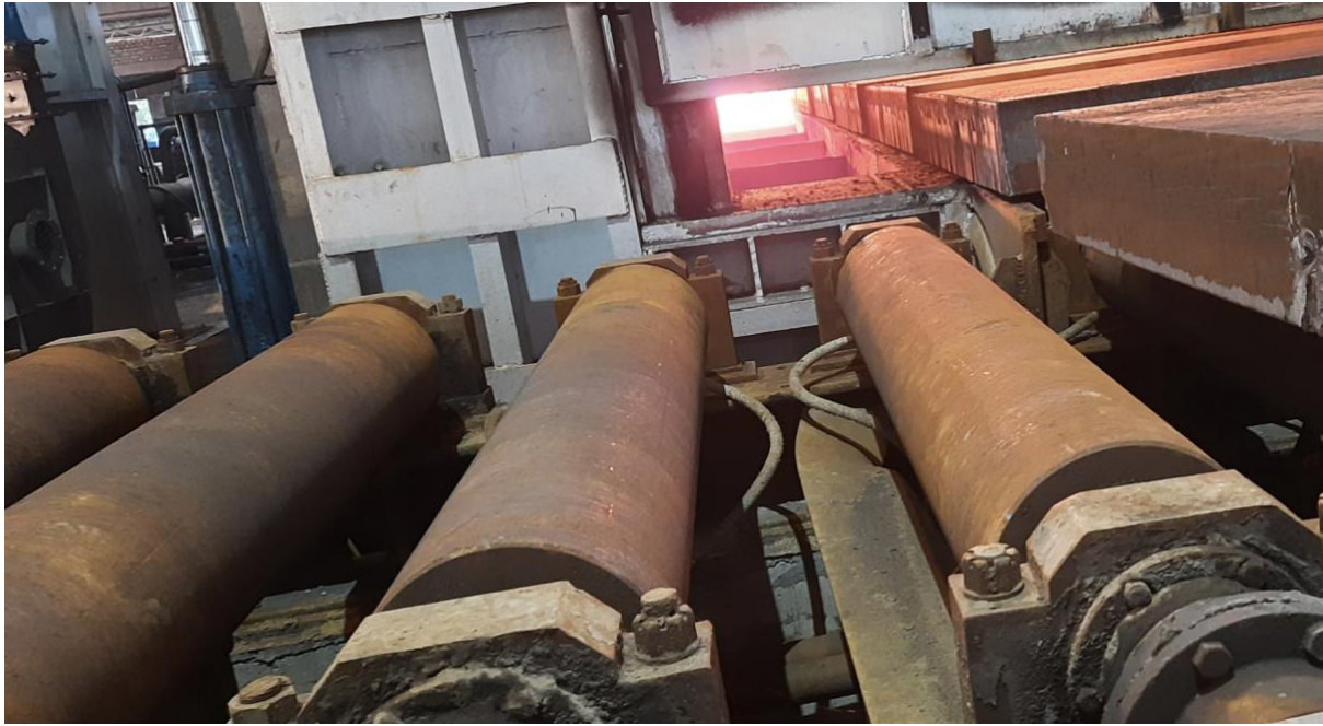
Figure 14 - Steel Slabs being 'charged' into RHF.
