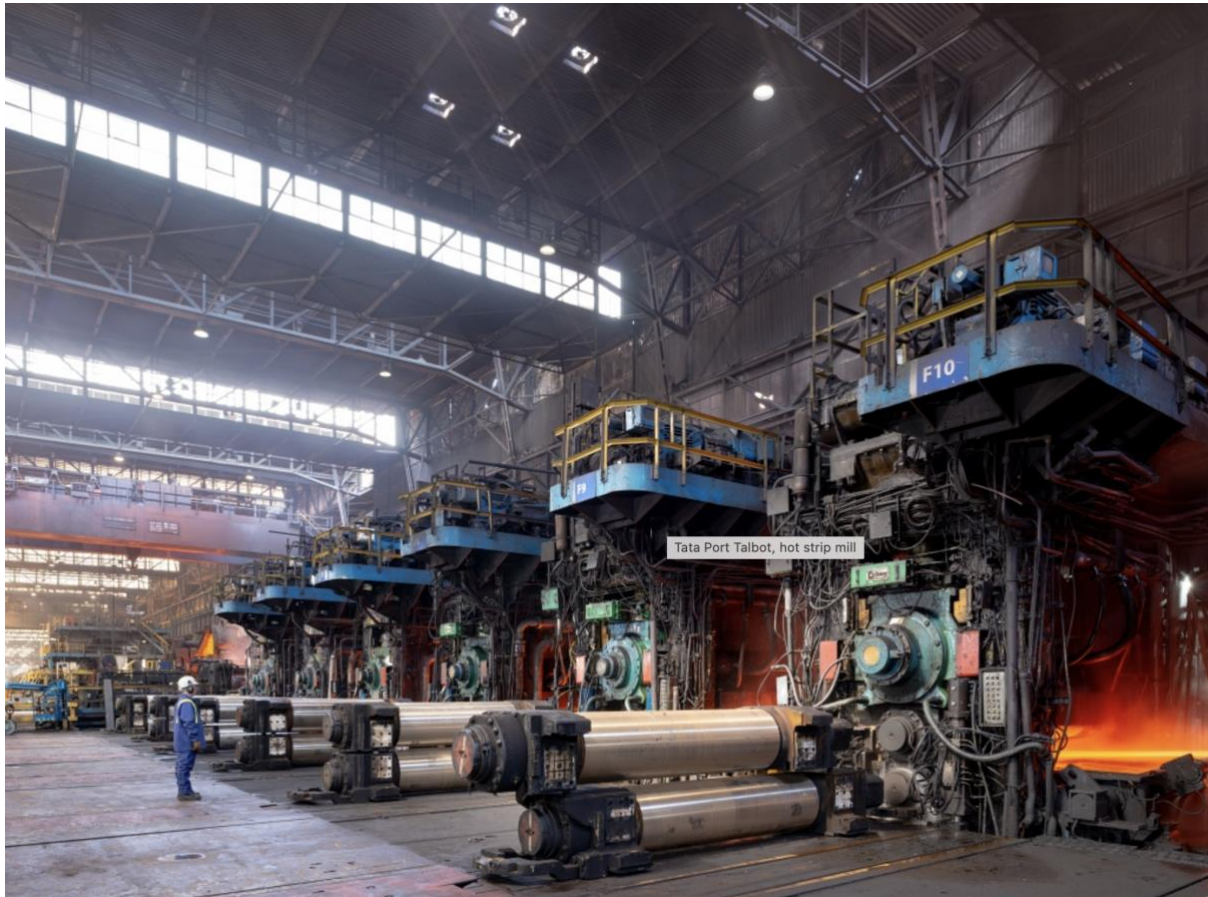
Figure 23 - Finishing Mill Stands, also showing new work rolls on the mill floor
