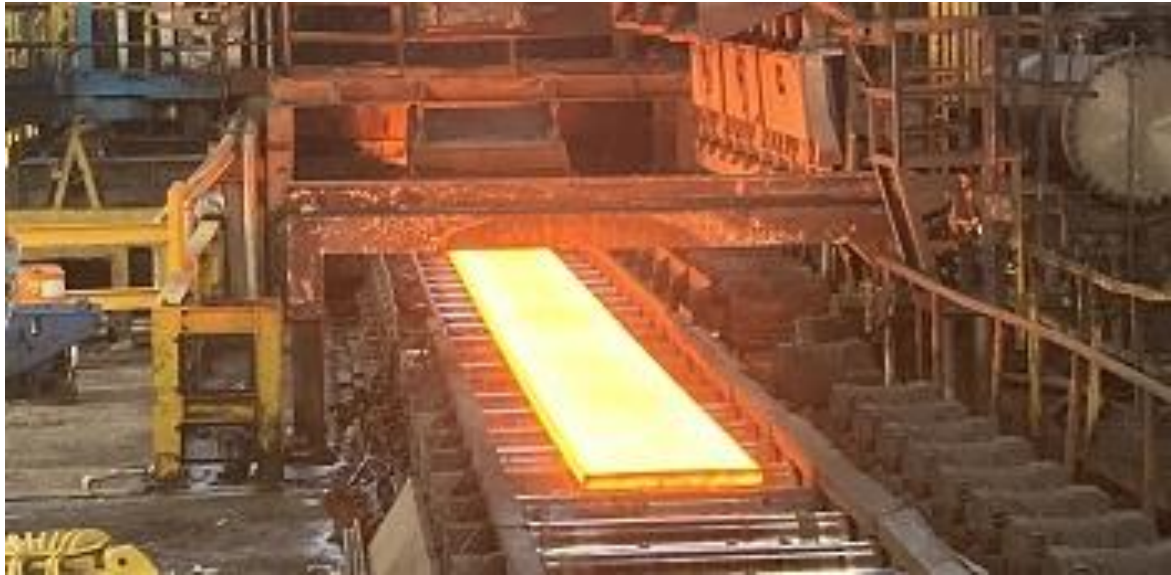
Figure 19 - Steel slab exiting the Reversing Rougher
