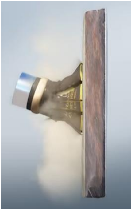
Figure 4: HESH round compressed against target, as shown in [7]
