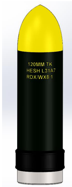
Figure 5: SolidWorks design of the external casing for the 120mm projectile for use in the simulation.
