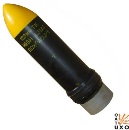
Figure 1: Image of a 120mm HESH L37A1 projectile from [3].
