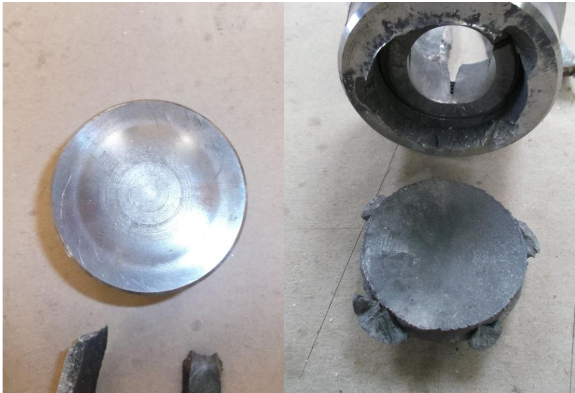
Figure 15 - End cap damage from firing 3 (left) and firing 1 (right)
