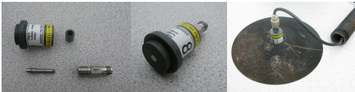
Figure 12 - Kistler Pressure Sensor, mounted in housing (right)
