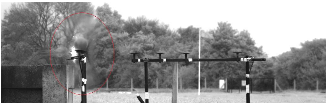
Figure 35 - Still from Lil' Gun firing @1ms, showing distortion of a primary blast wave, with initial reaction and dispersal of propellant
