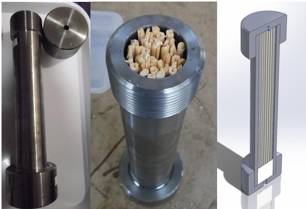
Figure 7 - Tube arrangement used in firings 1 and 2
