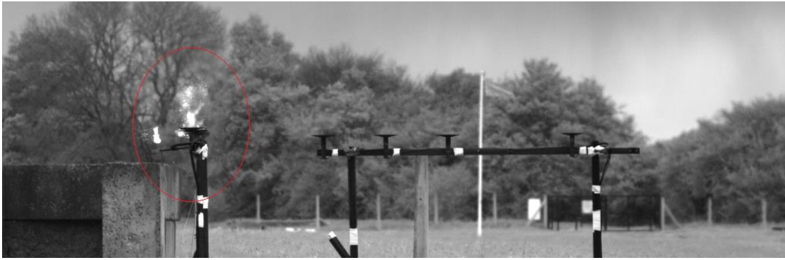
Figure 36 - Still from BL-C(2) firing @1.2ms, showing dispersal and burning of propellant away from the charge
