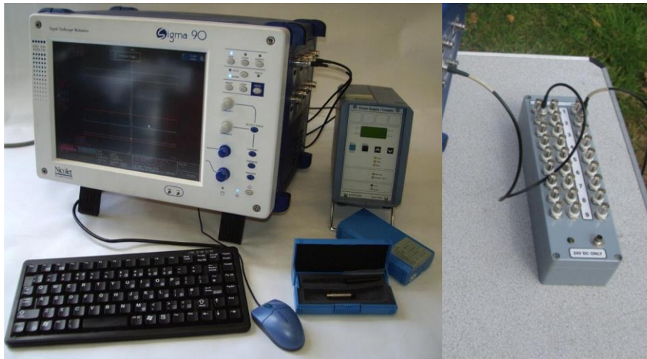
Figure 11 - Sigma 90 Digital Storage Oscilloscope used for data recording, with power supply unit (Right)
