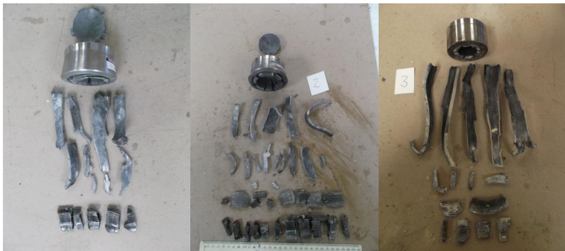
Figure 14 - Fragments Recovered from (L-R) firings 1 and 2 (propellant) and 3 (inert)
