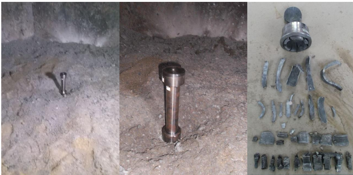
Figure 8 - Completed stage 1 charges in the containment building, with remaining fragments shown right
