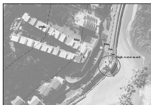
Figure 8: Impact on structures, influenced by distance from the high-water mark, building a is more likely to be damaged than building b, due to its location
