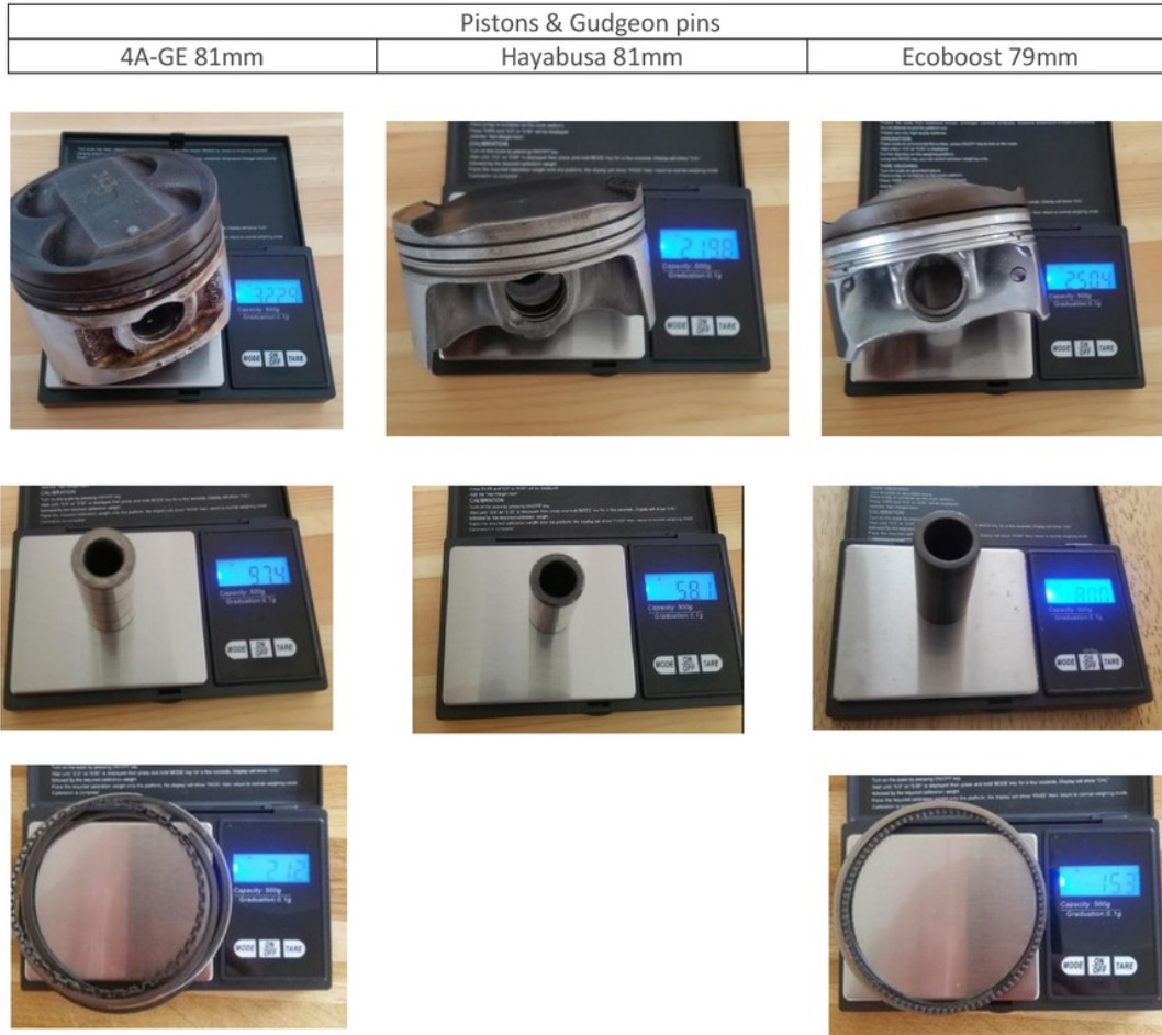
Figure 3-1 Piston, Gudgeon Pin & ring Mass including possible Hayabusa lightweight option (Evans, 2019)
