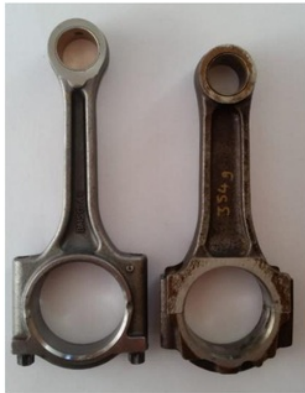
Figure 3-9 Ecoboost rod pictured left & 4A-GE or right. (Evans, 2019)
