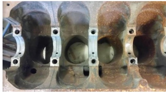
Figure 3-12 4A-GE crankcase. No machined areas and smaller space so 7A-FE & Ecoboost cranks will not spin. (Evans, 2019)
