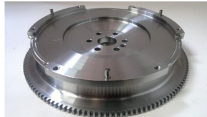
Figure 4-4 Ecoboost aftermarket Solid flywheel to replace the original dual mass flywheel. (ttvracing.com, 2019)
