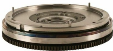
Figure 4-5 Actual DMF belonging to an Ecoboost. (ebay.co.uk, 2019)
