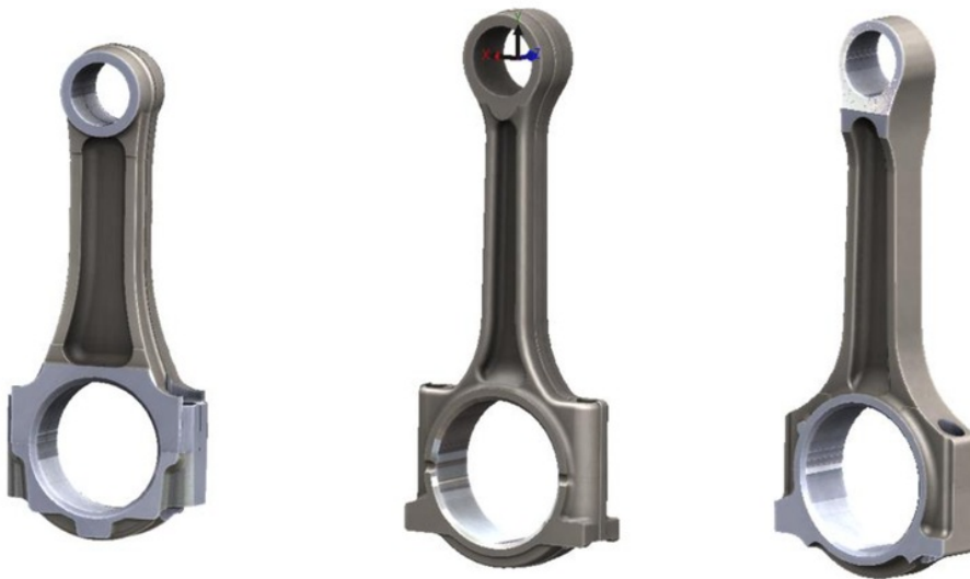
Figure 3-15 CAD Models of the conrods from left to right, 2 nd Gen 4A-GE, 1st gen Ecoboost, 2nd Gen Ecoboost. (Evans, 2019)
