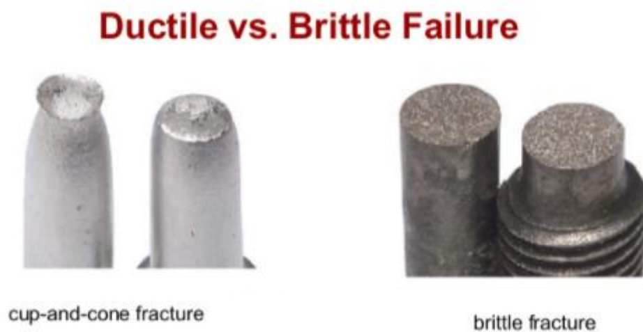
Figure 13- Ductile vs Brittle Fracture (Engineering Stack Exchange, 2021)
