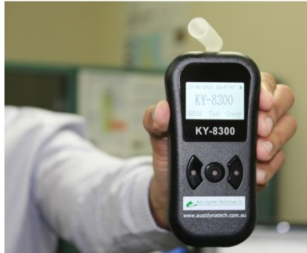
Figure 6: Example of handheld breathalyser device fitting in a human hand
