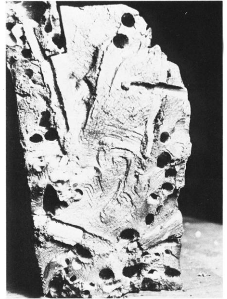
FIG. 2. Kyrenia ship, a lateral break in the keel, showing square side pegs and a fragment of garboard attached to the keel by a mortise-and-tenon joint. (Photo Robin C. M. Piercy)
