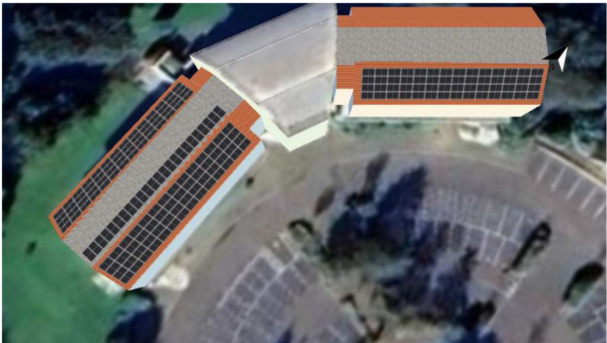
Figure 8: Solar Panel Layout
