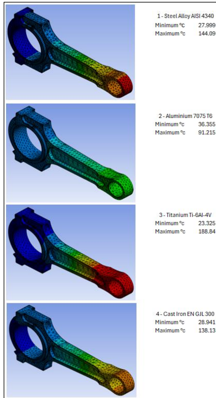
Figure 14: showing the temperature profiles of each material based on expected temperatures
