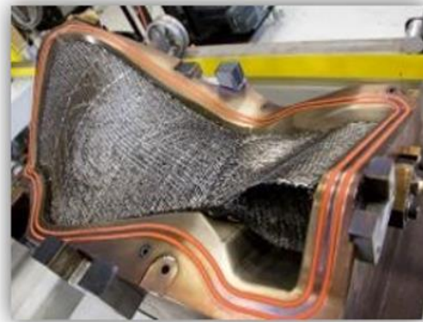
Figure 5: Safran LEAP Fan Blade in mould post RTM (Fehrm, 2016))
