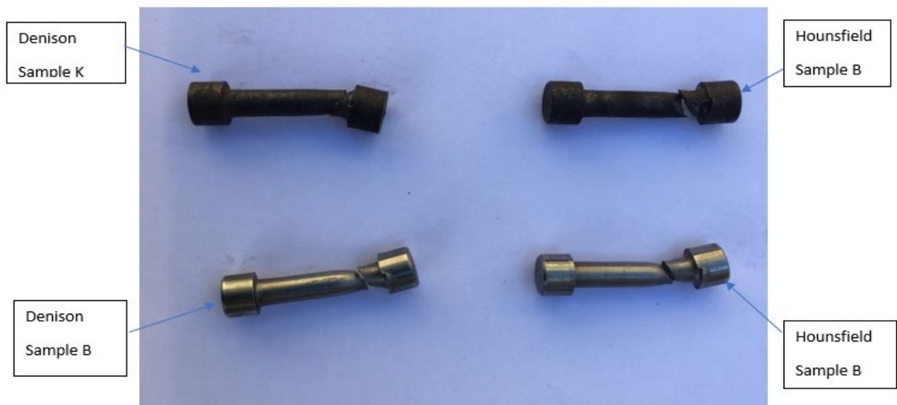
Figure 27 shows samples broken from near the specimen's shoulder, created by the old collet from both machines.
