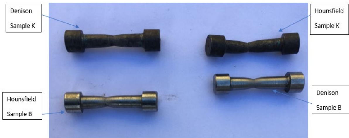
Figure 26 shows samples broken from the middle created by the new collet from both machines.
