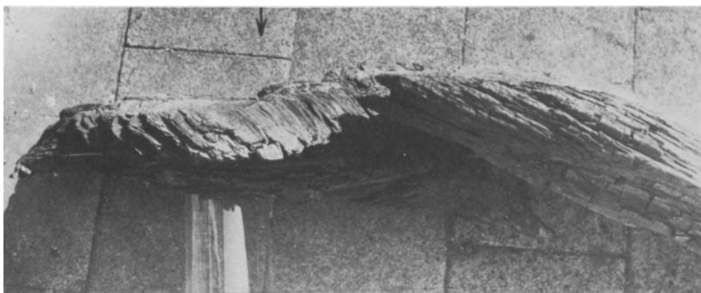
Figure 16. Bruges boat: side view of floor-timber (Fig. 10, no. 9), the arrow indicating the suggested reverse clinker construction.
