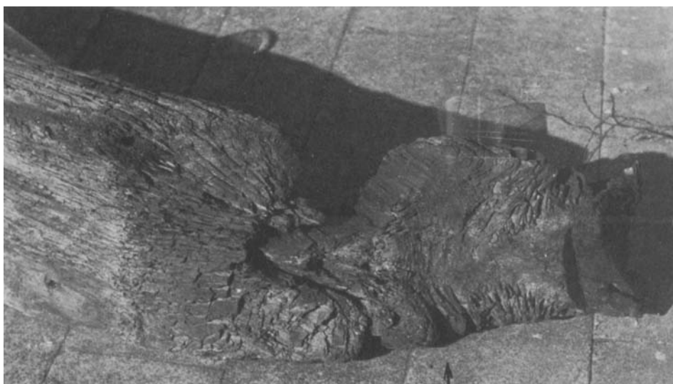
Figure 17. Bruges boat: underside view of the timber shown in Fig. 16, the arrow indicating the suggested reverse clinker construction, and showing that the 'step' in the rib is not continuous across the floor-timber. At the extreme right end is a modern saw cut.
