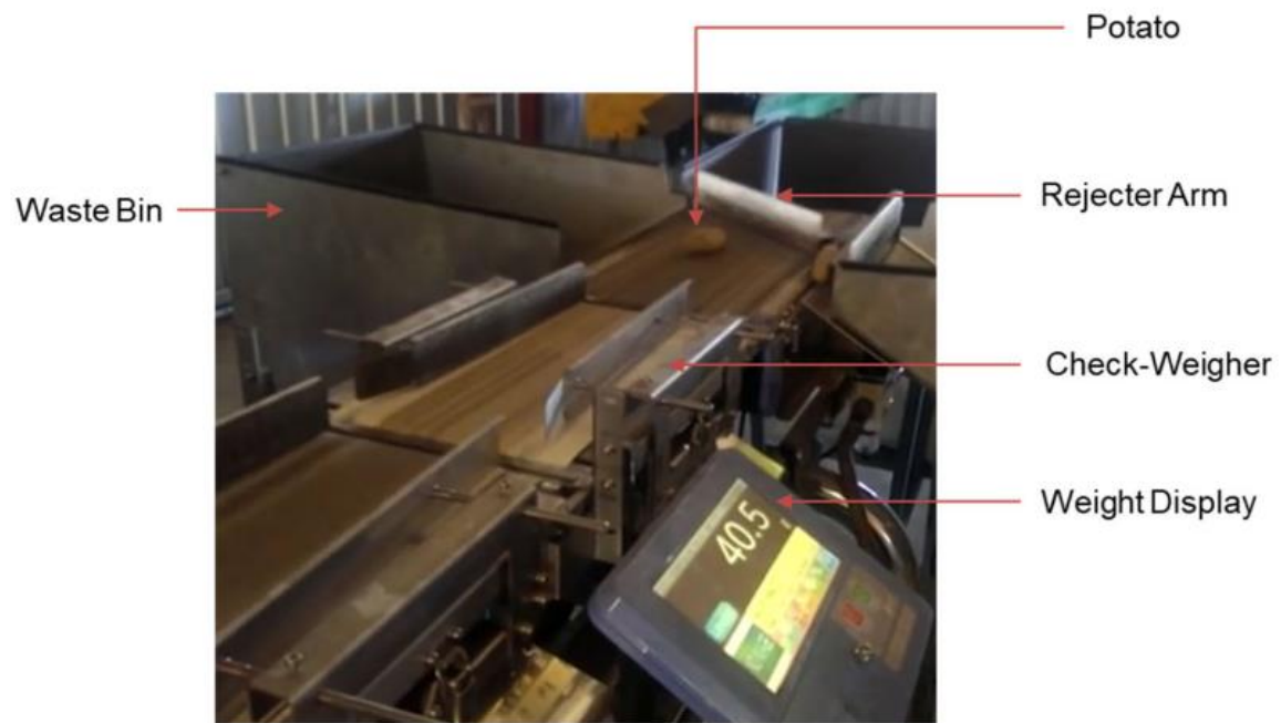
Figure 2 explains the check-weigher systems (Jagtap, S. et al. 2019).
