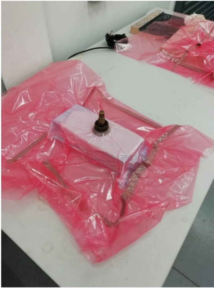
Figure 5 - Vacuum bag ready to be opened
