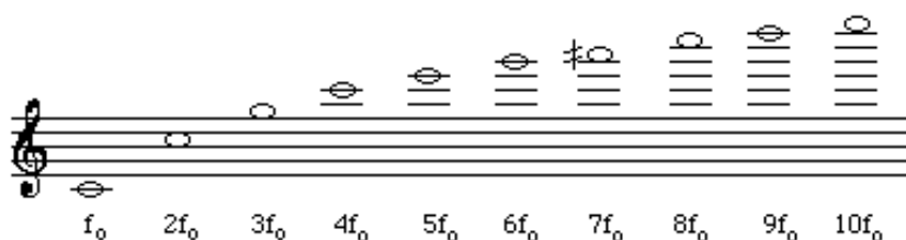
Figure 4 - harmonic pitches of a flute from C4
