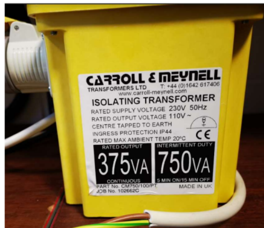
Appendix Image 2 - 240v-110v Transformer
