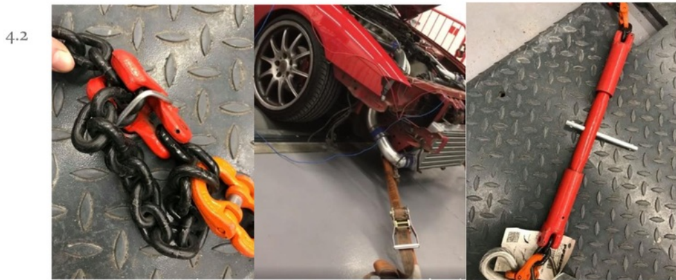
Figure 1 - Strapping the Car to the Dynamometer
