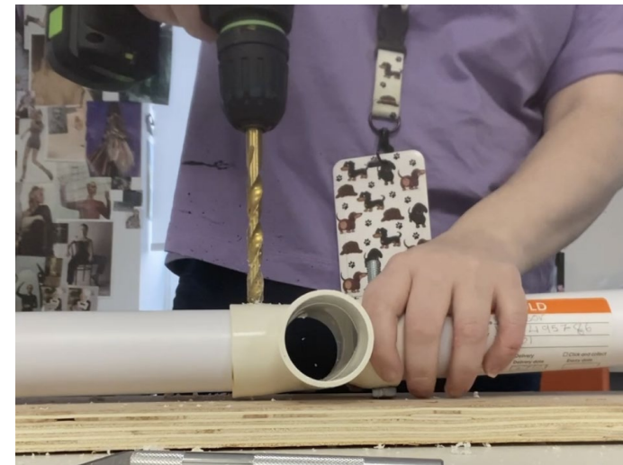
Drilling holes for Bolts for Reusability/Adaptability
