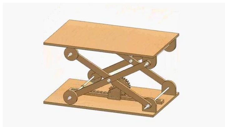
Figure 17: Image showing the 2 nd lifting mechanism idea.
