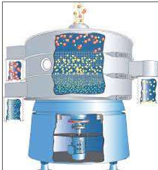
Figure 3 - Schematic of Vibratory Screening, Courtesy of, (Kay, 2010)
