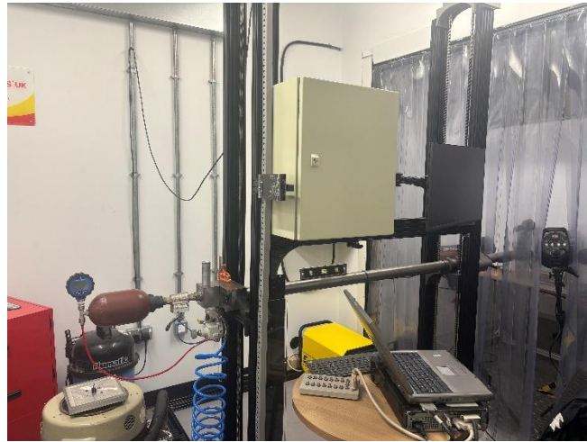
Figure 2: Image showing stone chip simulator .
