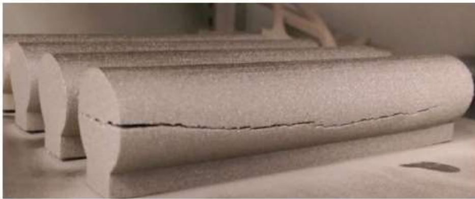
Figure 7 - Cracking and Distortion (Renishaw, 2023)
