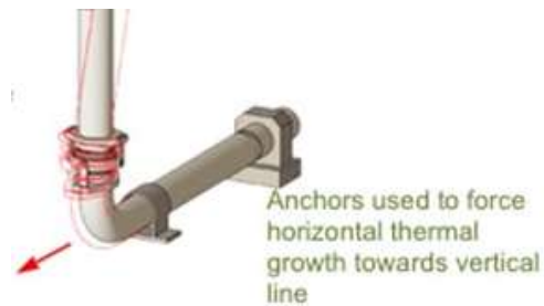
Figure 3 - Anchor Directing Thermal Growth (Pipingtech, 2023)
