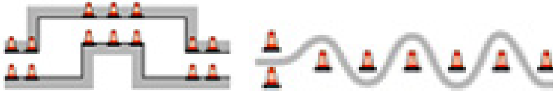
Figure 6: Simulator Manoeuvres: (Left) Double Lane Change, (Right) Slalom (OXTS, 2012).
