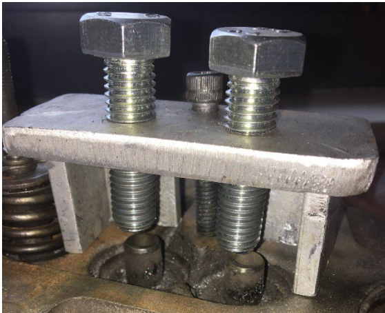
FIGURE 41: VALVE TOOL ON TOP OF CYLINDER HEAD
