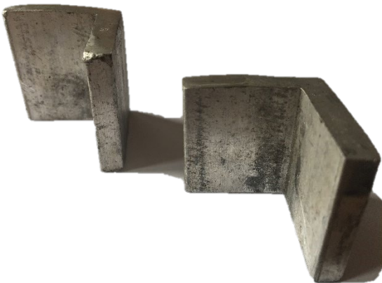
FIGURE 38: ALUMINIUM LEGS FOR VALVE OPENING TOOL
