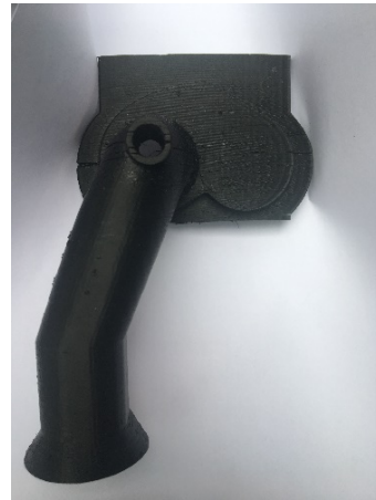
FIGURE 102: BOTTOM VIEW OF FLANGED PORT
