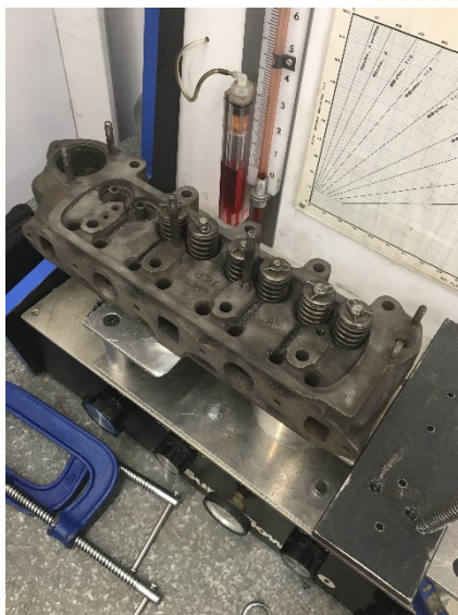
FIGURE 48: SITTING THE HEAD ON THE ADAPTOR PLATE
