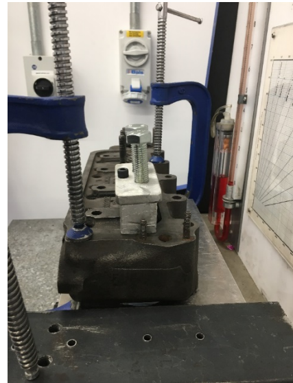
FIGURE 50: VALVE OPENING TOOL FROM THE SIDE
