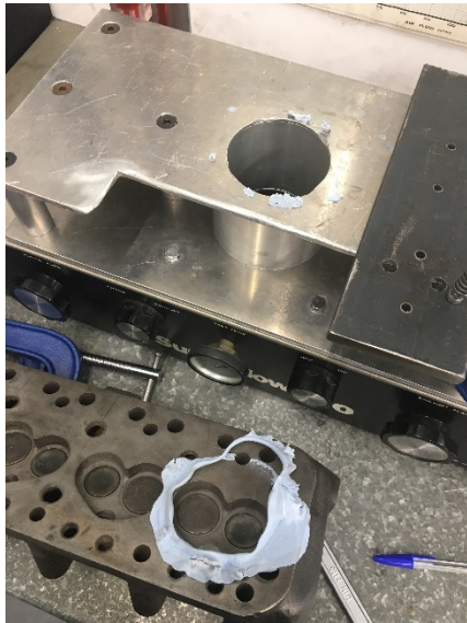
FIGURE 45: CREATING A SEAL ON THE CYLINDER HEAD
