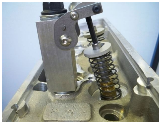
FIGURE 25: TYPICAL VALVE OPENING TOOL
