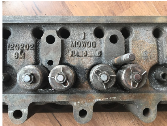
FIGURE 24: IMAGE SHOWING LACK OF THREADED HOLES TO BOLT INTO HEAD
