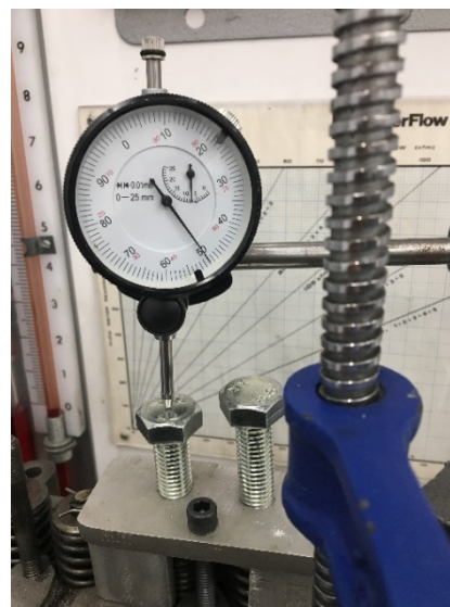
FIGURE 54: DTI WITH VALVE OPEN 0.5MM
