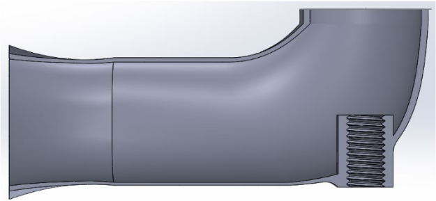
FIGURE 121: PORT 6 INCREASED SHORT TURN RADIUS
