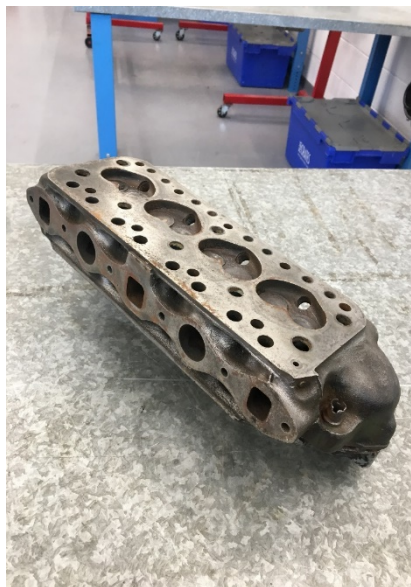
FIGURE 20: 12G202 PORTS AND CHAMBERS
