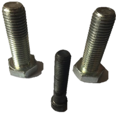
FIGURE 400: SECURING BOLT AND BOLTS USED TO PUSH DOWN VALVE
