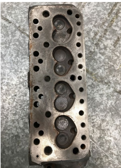
FIGURE 18: 12G202 COMBUSTION CHAMBERS
