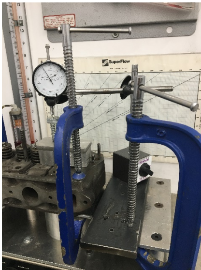
FIGURE 52: ADDING THE DTI GAUGE
