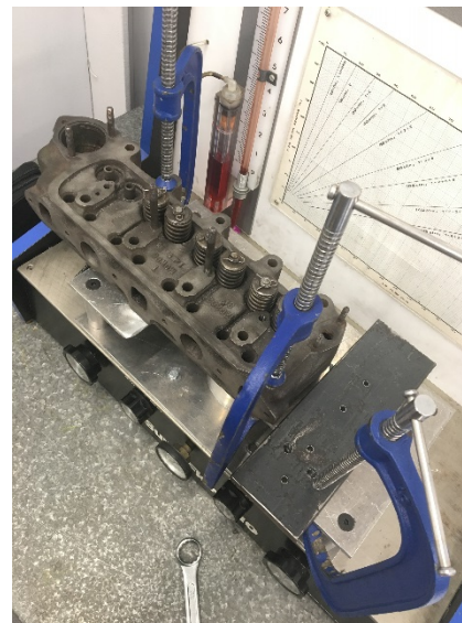
FIGURE 47: CLAMPING THE CYLINDER HEAD DOWN
