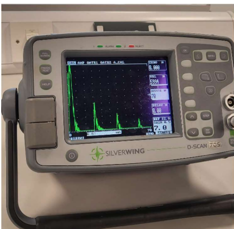
Figure 1-9: Backwall Reflections on Oscilloscope
