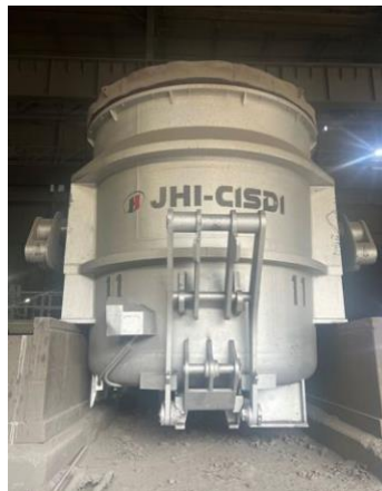
Image 1. Teeming Ladle at TATA Steel, Port Talbot
