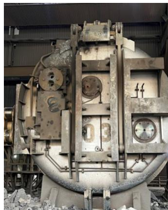
Image 3. Bottom of Ladle / Tipping Gear
