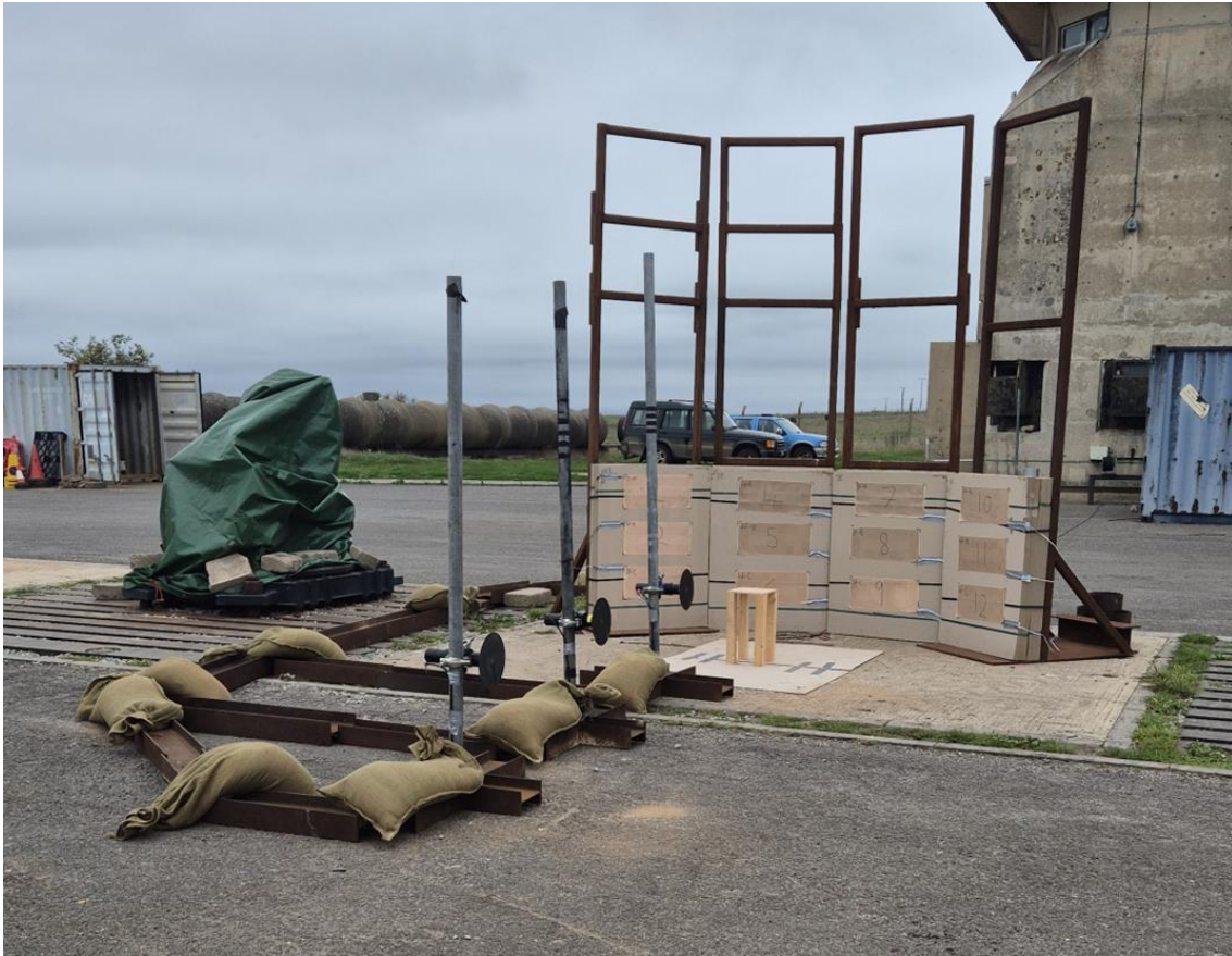
Figure 2-1 - Small Fragmentation Arena Trial Used to Identify an Unknown Munition
