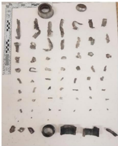
Figure 4-7 - Natural and Preformed Fragmentation Comparison [9, 16]
