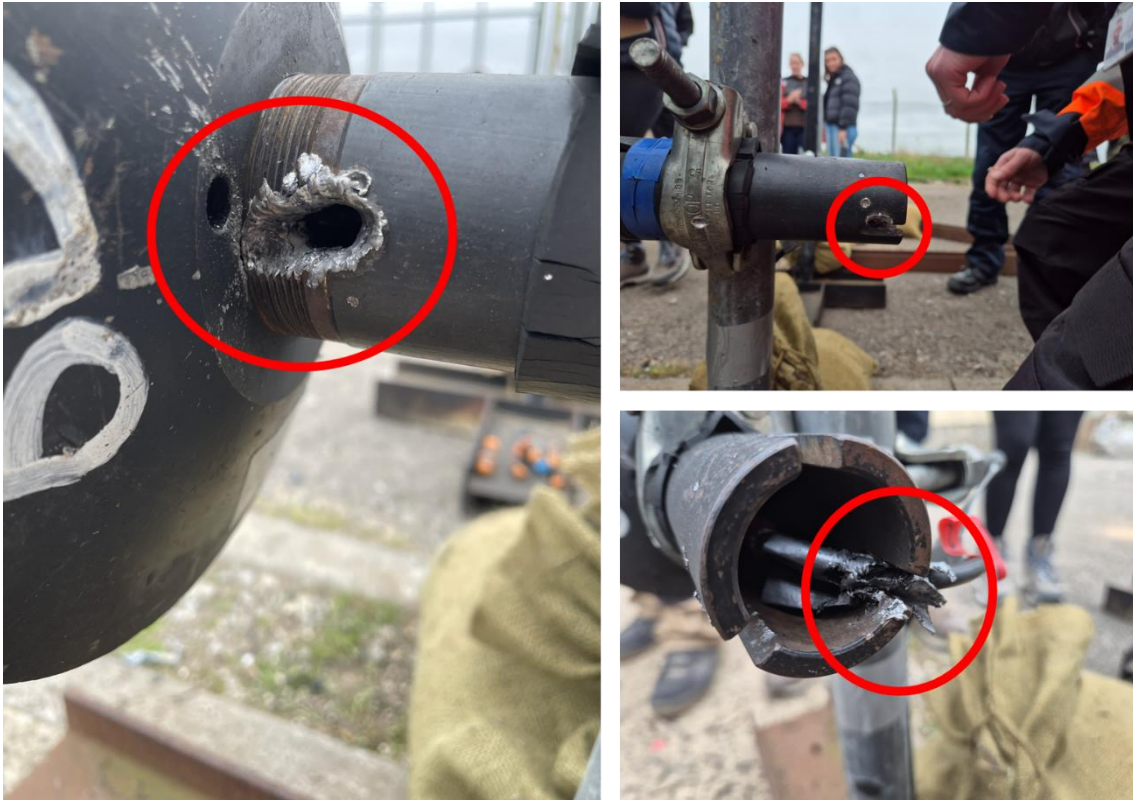
Figure 3-2 - Gauge One - Fragmentation Damage
