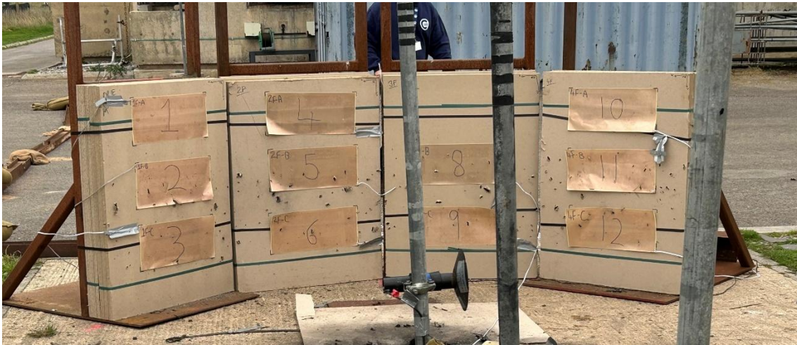
Figure 3-4 - Fragmentation Strikes Captured on Strawboard
