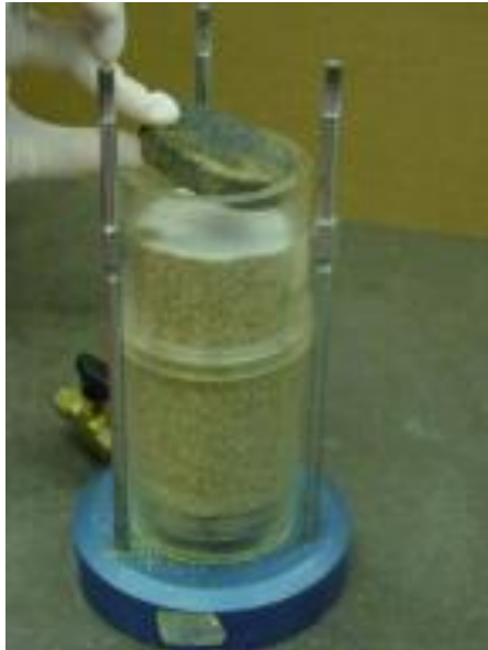
Figure 8 – Soil inserted with graded gravel filter on top of permeameter (Reddy, n.d.)
