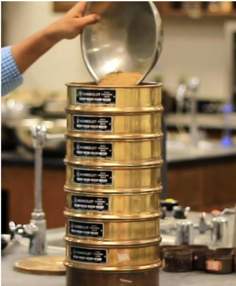
Figure 10 – Pouring our sample soil into the sieve (Hossain, Islam, Badhon and Imtiaz, 2022)
