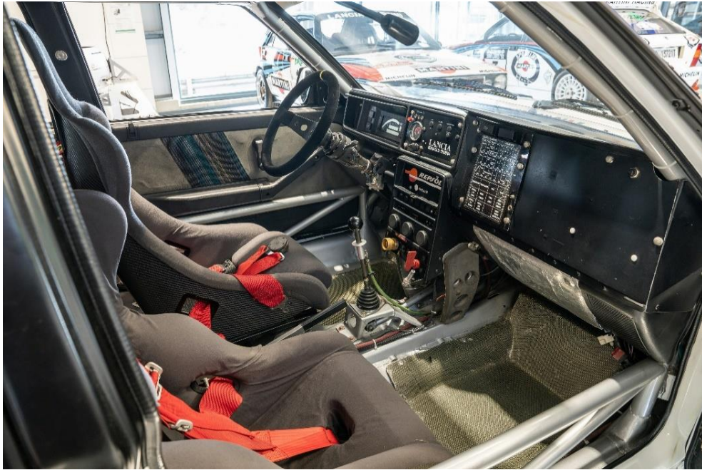
Figure 6. Interior of the 1991 Group A Lancia Delta HF with additional longitudinal struts
