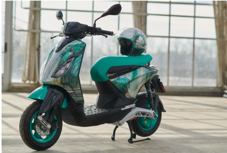
Figure 6 - The Piaggio One is an electric scooter aimed for city use and is driven by a hub motor in the rear wheel. (Attwood, 2022)
