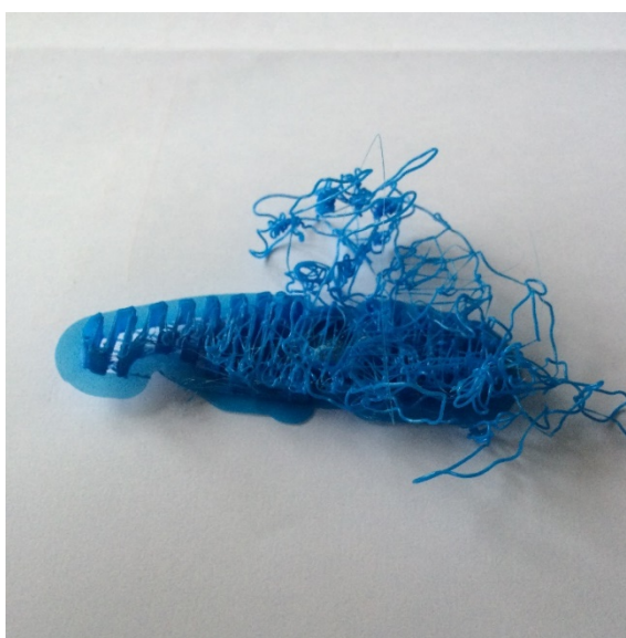
Figure 5. An Example of a Failed Print, in This Case the Part Became Detached from The Build Plate Because the Bed Temperature Was Too Cool.
