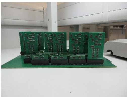
Figure 26. Constructed reversible adder backplane filled with logic gates.
