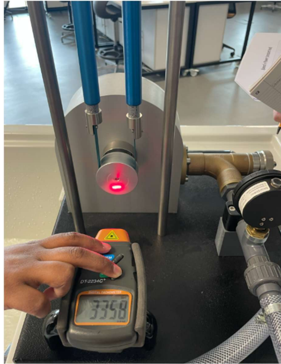
Figure 3. Rear view of the Pelton turbine test rig showing the fixed laser tachometer used to measure rotational speed at the belt pulley.
