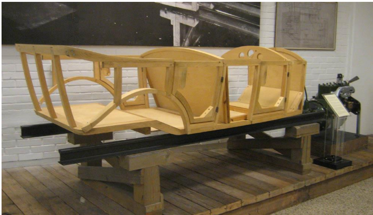
Figure 1- Conventional Coachwork frame ( https://en.wikipedia.org/wiki/Weymann_Fabric_Bodies )
