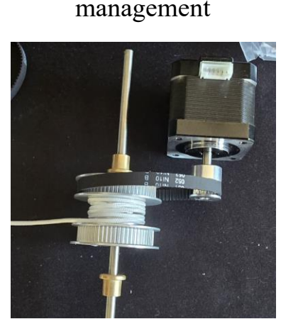
Figure 8: Stepper Motor 2 excess string management
