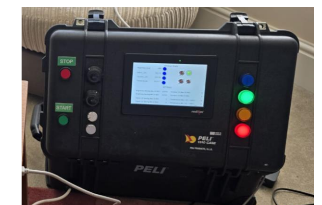
Figure 11: Peli Case showing Buttons, LEDs and HMI Screen
