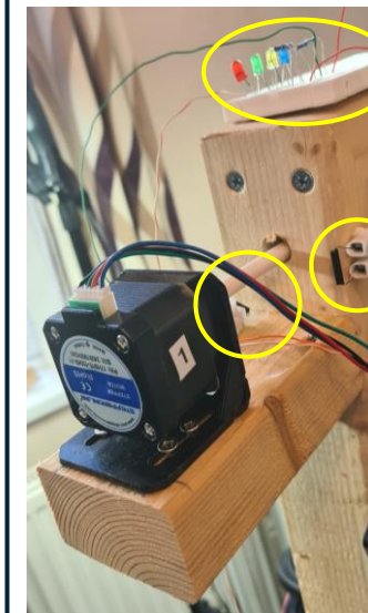
Figure 6: Stepper Motor 1, controlling blind angles
