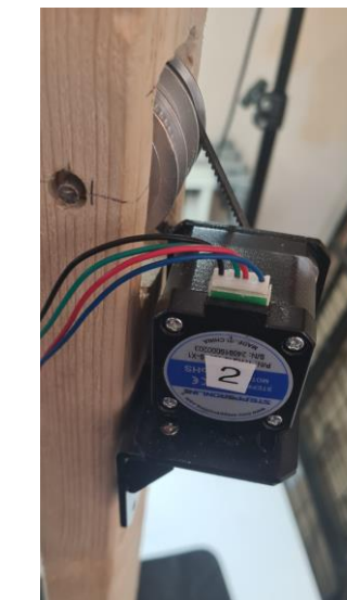
Figure 7: Stepper Motor 2, controlling blind height
