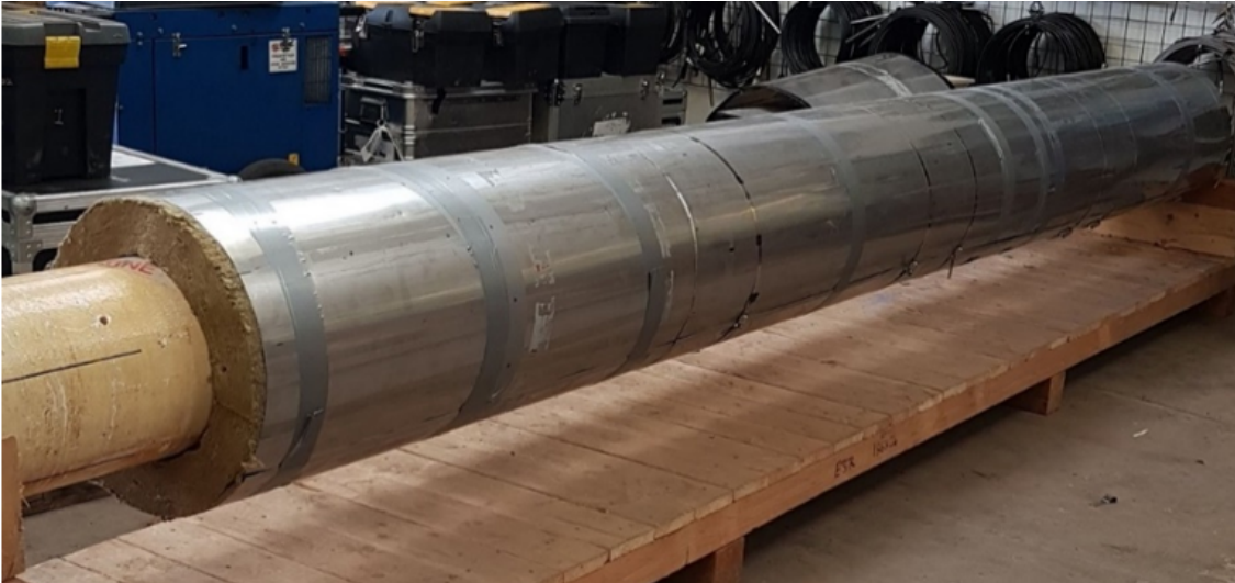
Figure 3.2: Pipe under insulation and cladding
