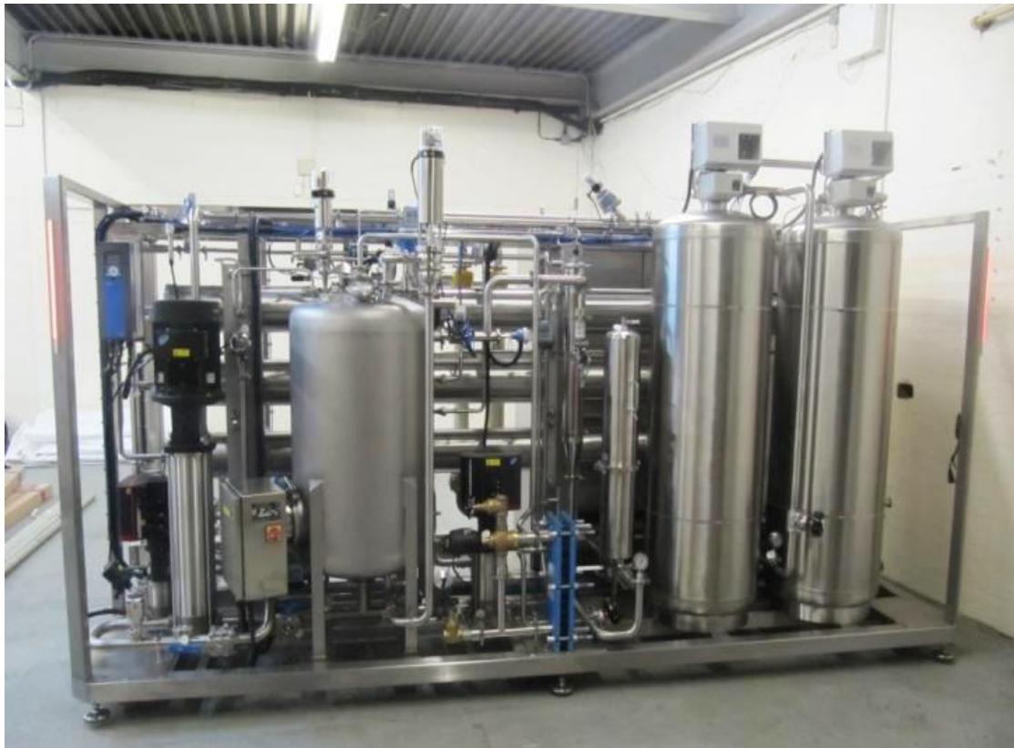
Figure 52 Orion 4000 skid manufactured from 300 series stainless steel
