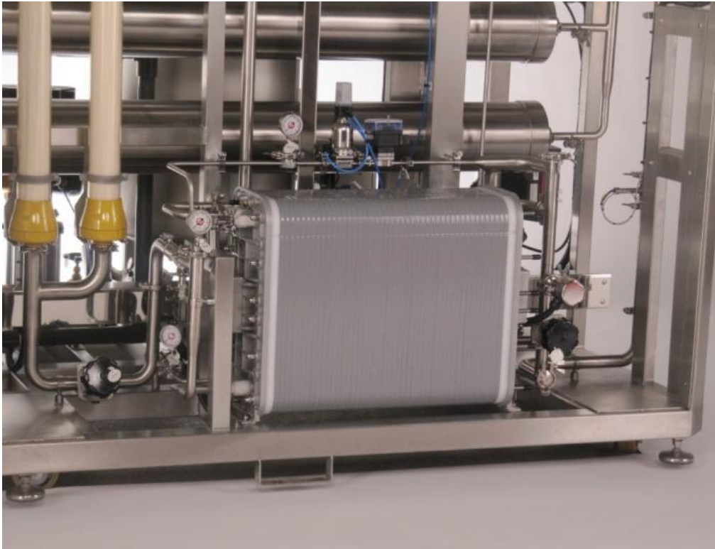
Figure 54 CEDI manufactured from stainless steel
