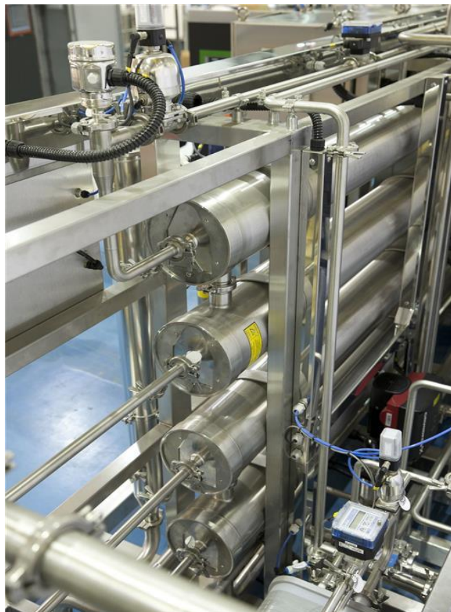
Figure 53 Reverse osmosis membrane housing manufactured from stainless steel
