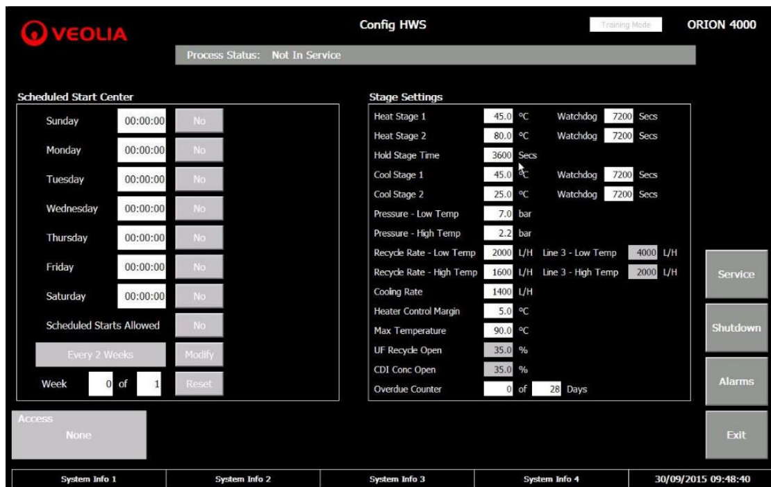
Figure 50 Hot water sanitisation configuration screen
