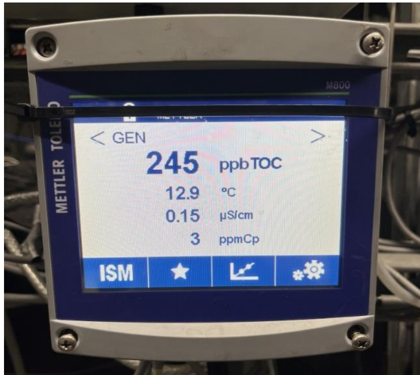
Figure 60 Orion continuous in-line monitoring. Measuring total organic carbon, temperature, conductivity, and parts per million
