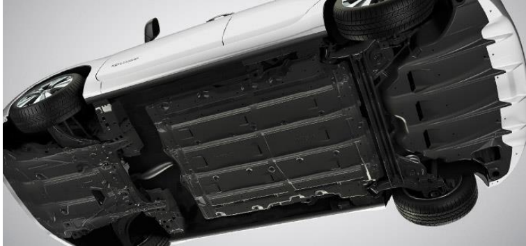
Figure 2-6 Rally Car underbody Diffuser (Nissan, 2017)
