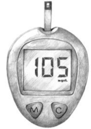
This is a blood glucose meter with a test strip inserted (National Institute of Diabetes and Digestive and Kidney Diseases, 2026)
