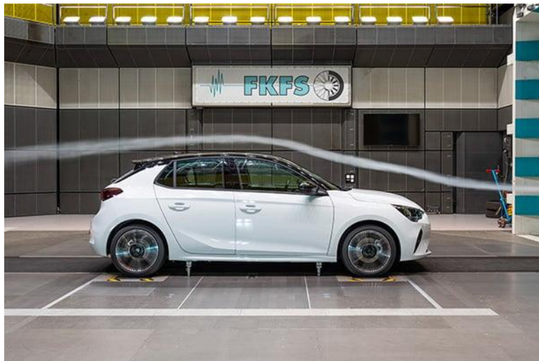
Example of the Vauxhall Corsa getting tested in a wind tunnel. (nationwide vehicle contracts)
