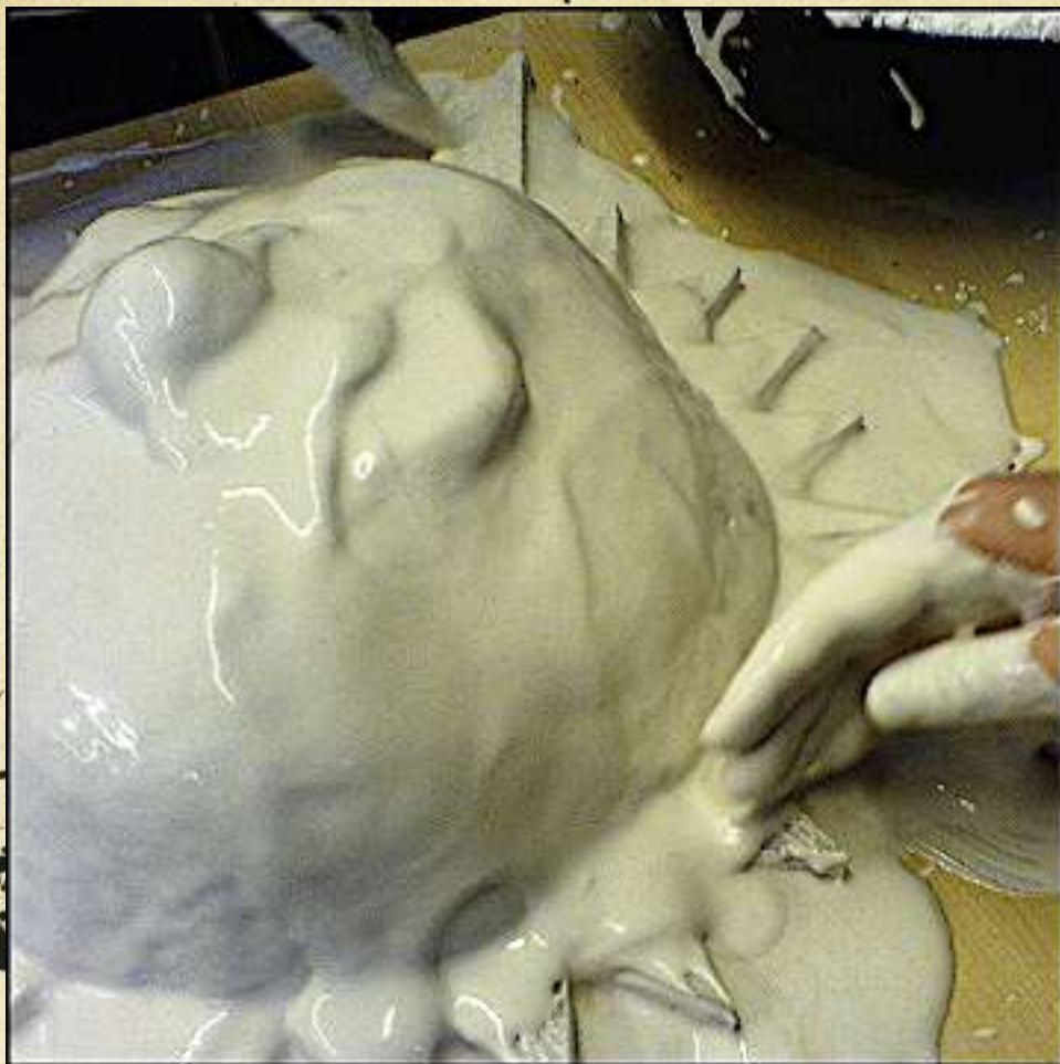
First layer of fine casting Plaster flicked onto model
