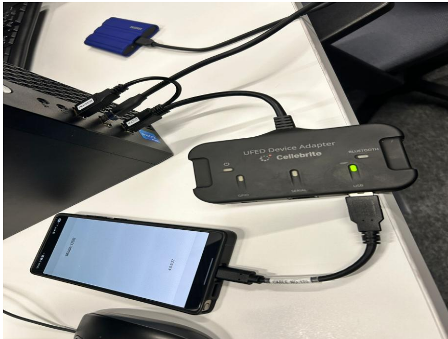
Figure 2: Samsung S25 Ultra connected to UFED Device Adapter via Cable No. 170
