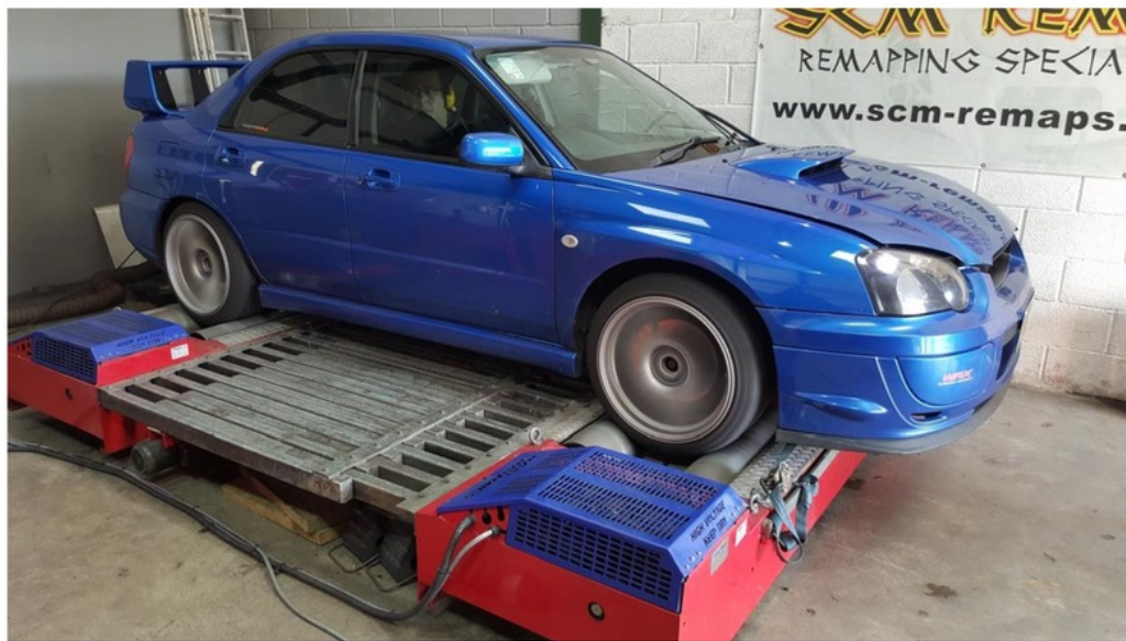
Figure 12 Dyno featuring double roller (SCM Remaps, 2019)
