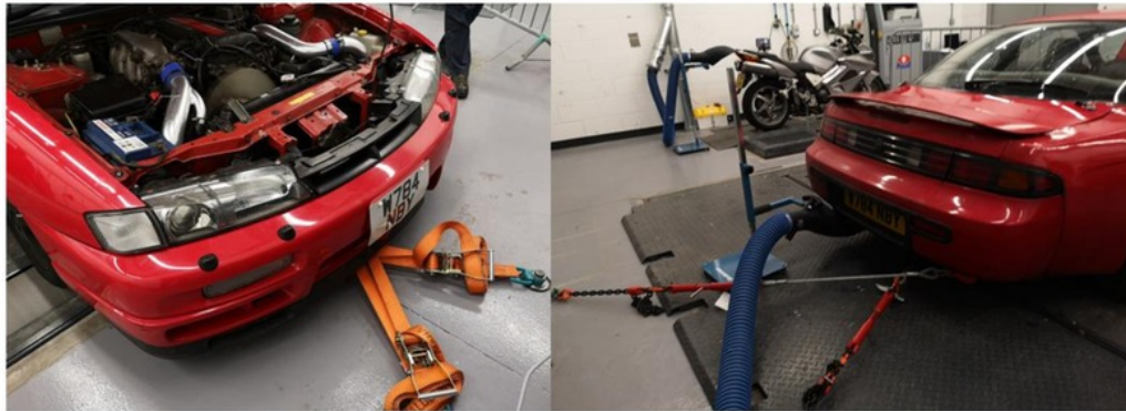
Figure 16 Photograph of S14 securing points on dyno
