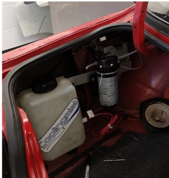
Figure 22 Photograph showing Water/Methanol Installation in vehicle
