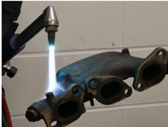
Figure 18 Photo of exhaust manifold being welded
