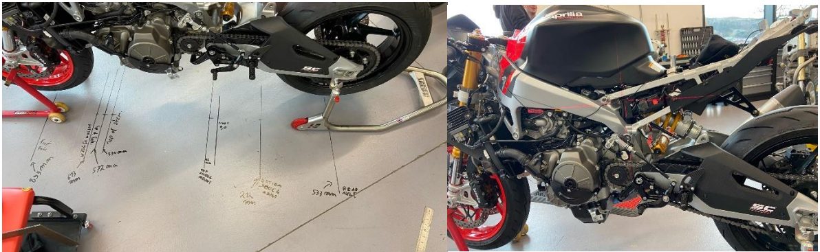
Figure 8: Frame Points Location Measurement (Iatrakis, 2024)
