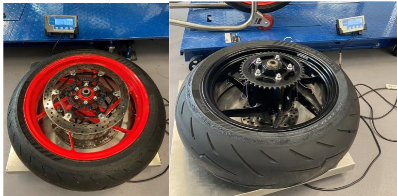
Figure 25: RS660 Wheel weight measuring (Iatrakis, 2024)
