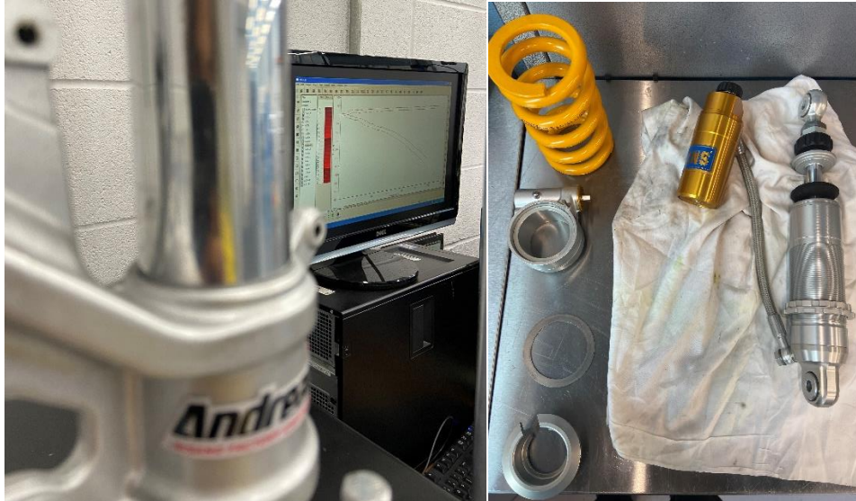
Figure 4: Andreani Fork on Damper Dyno & Spring/ shock disassembled for the Damper Dyno. (Iatrakis, 2023)
