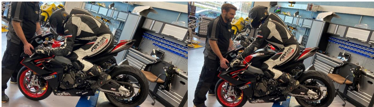
Figure 3: Rider tucked (Left) & Rider Upright (Right) CoG Measurement (Iatrakis, 2023)
