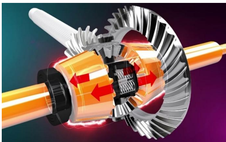
Figure 16: Cone Clutch LSD Operation (Autodata Training, 2019).
