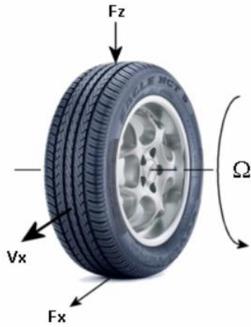
Figure 8: (Left) Longitudinal Tyre Model Diagram (Mathworks [2], 2025), (Right) Pacejka Longitudinal Force Against Slip Angle Graph Demonstration- Modified from (Vogel, 2021).
